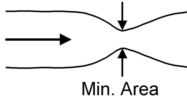
For steady adiabatic flow:  $V = \sqrt{2C_p(T_0 - T)}$
