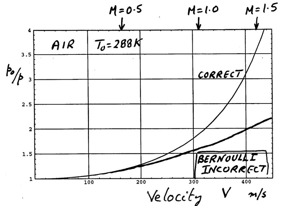
Bernoulli's Equation is **NOT** correct for the flow of gases. It should only be used where the Mach number is less than 0.3, i.e. where the effects of compressibility are small.
