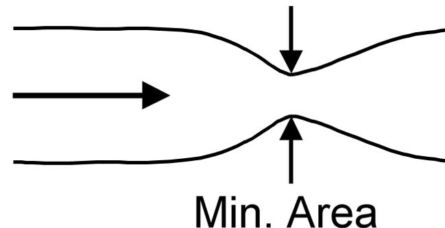
It is not normally worthwhile fitting a con-di nozzle to a subsonic civil aircraft as the exit jet velocity will only be slightly supersonic. (Unconstrained expansion.)
