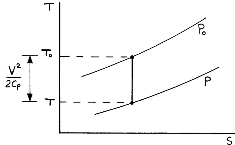
In carrying out the cycle analysis, for example finding the work or heat transfer, in a gas turbine, it is the **stagnation** quantities which should be used.
