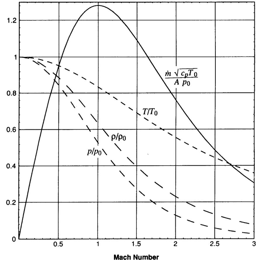
Figure 6.2. One-dimensional flow of a perfect gas,  $\gamma = 1.4$
